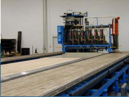
The Semi-trailer floor assembly machine designed and built by GT Automation locates the I beam cross members in an adjustable fixture which accommodates various trailer widths and beam spacing. Typically it will accommodate up to three widths and beam spacings. The fixture clamps the beams and squeezes the wood or aluminum floor. It can also handle a hybrid wood and aluminum floor.
