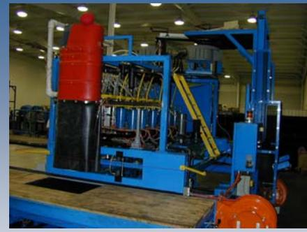
Our machine moves over the fixtured floor guided by a rail system and positioned by an integrated AC servo drive unit and encoder. The PLC retains location information in the case of power loss.
